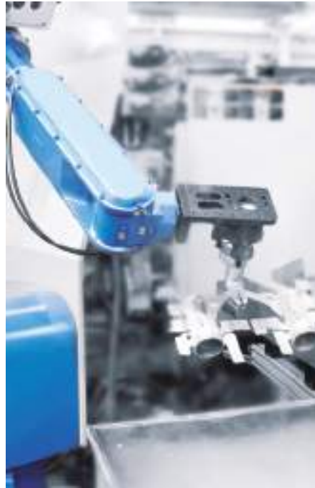
Parallel Gripper MCHJ for die casting gripping application.
