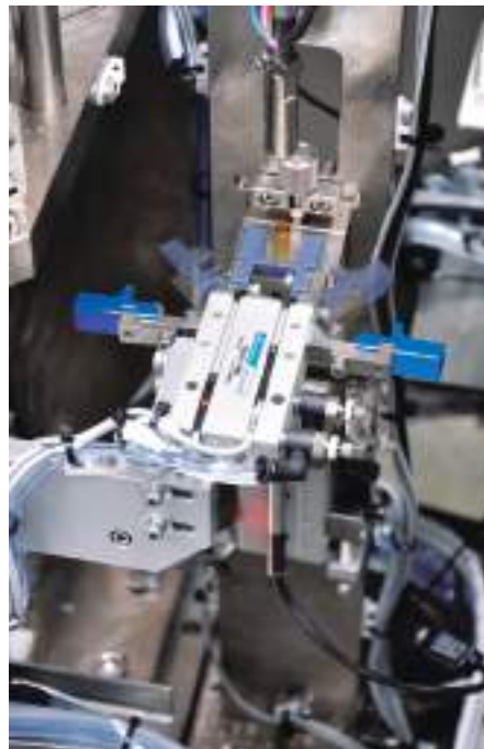
Angle gripper MCHY for assembly part clamping application.
